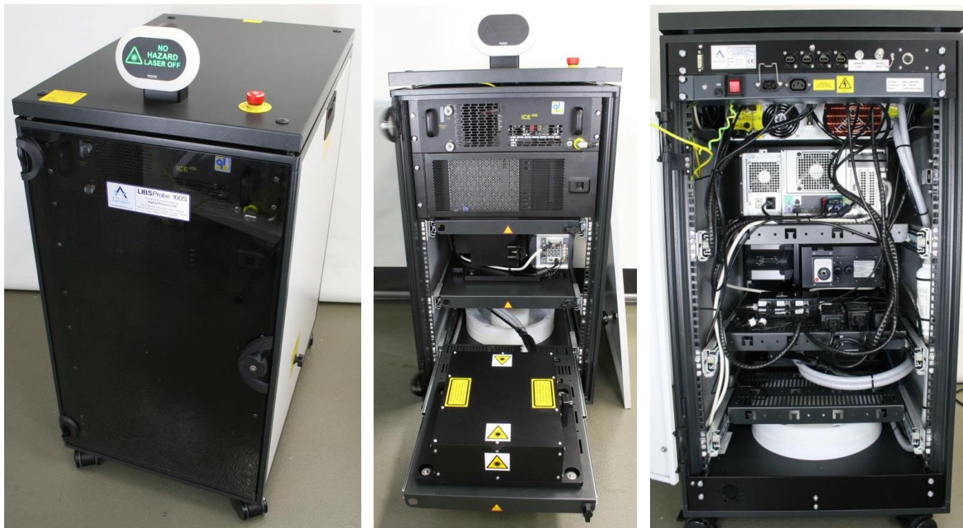
Images of the LIBS instrument rack unit housing the laser, the optical spectrograph, fibre launch optics and system computer
