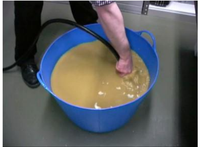
Identifying materials submerged in clean and turbid water using a submersible FO-LIBS probe
