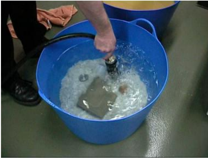
Identifying materials submerged in clean and turbid water using a submersible FO-LIBS probe
