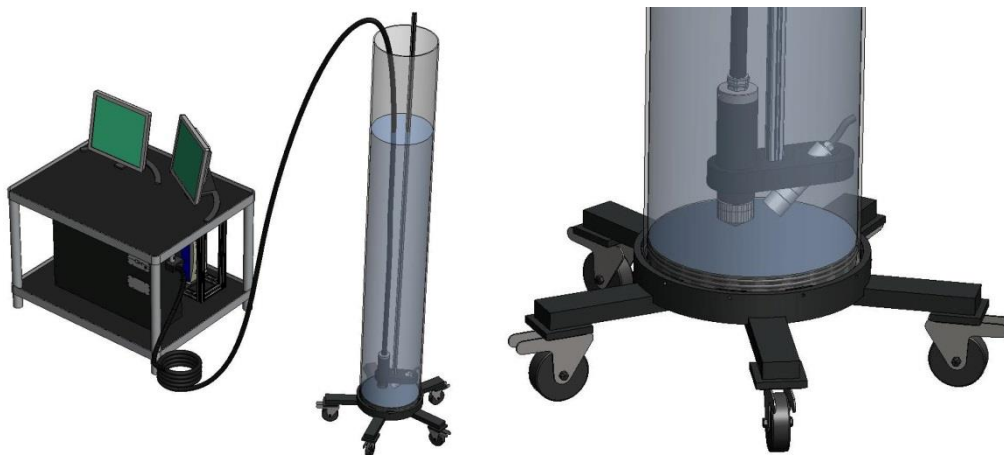
Submersible FO-LIBS probe and water-filled transparent polycarbonate tube, 350 mm diameter and 2 metres height
