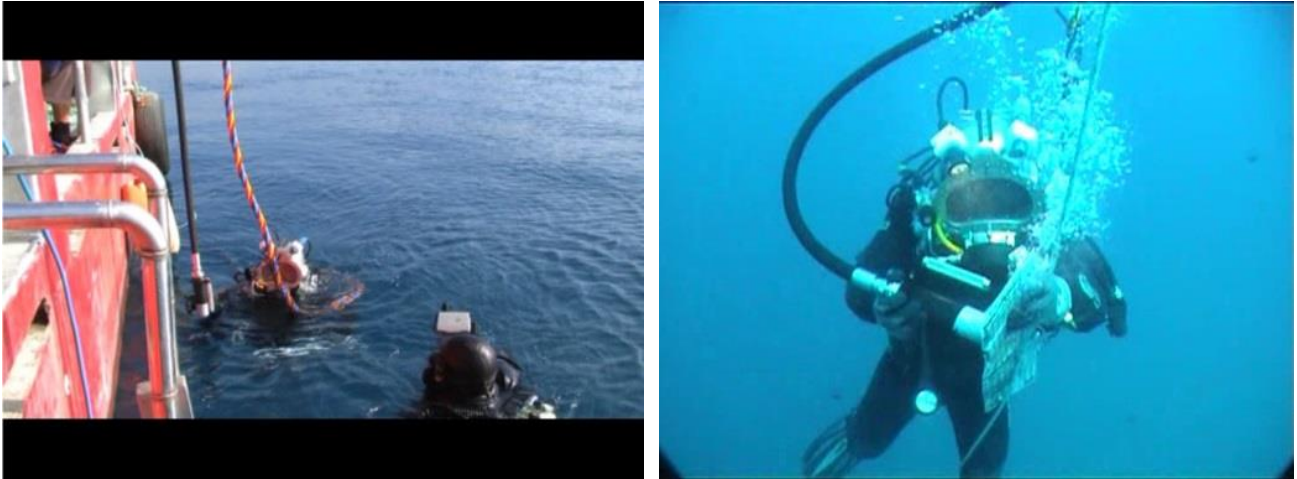
Deployment of the submersible FO-LIBS probe at depths of up to 30 metres (images courtesy of University of Malaga)
