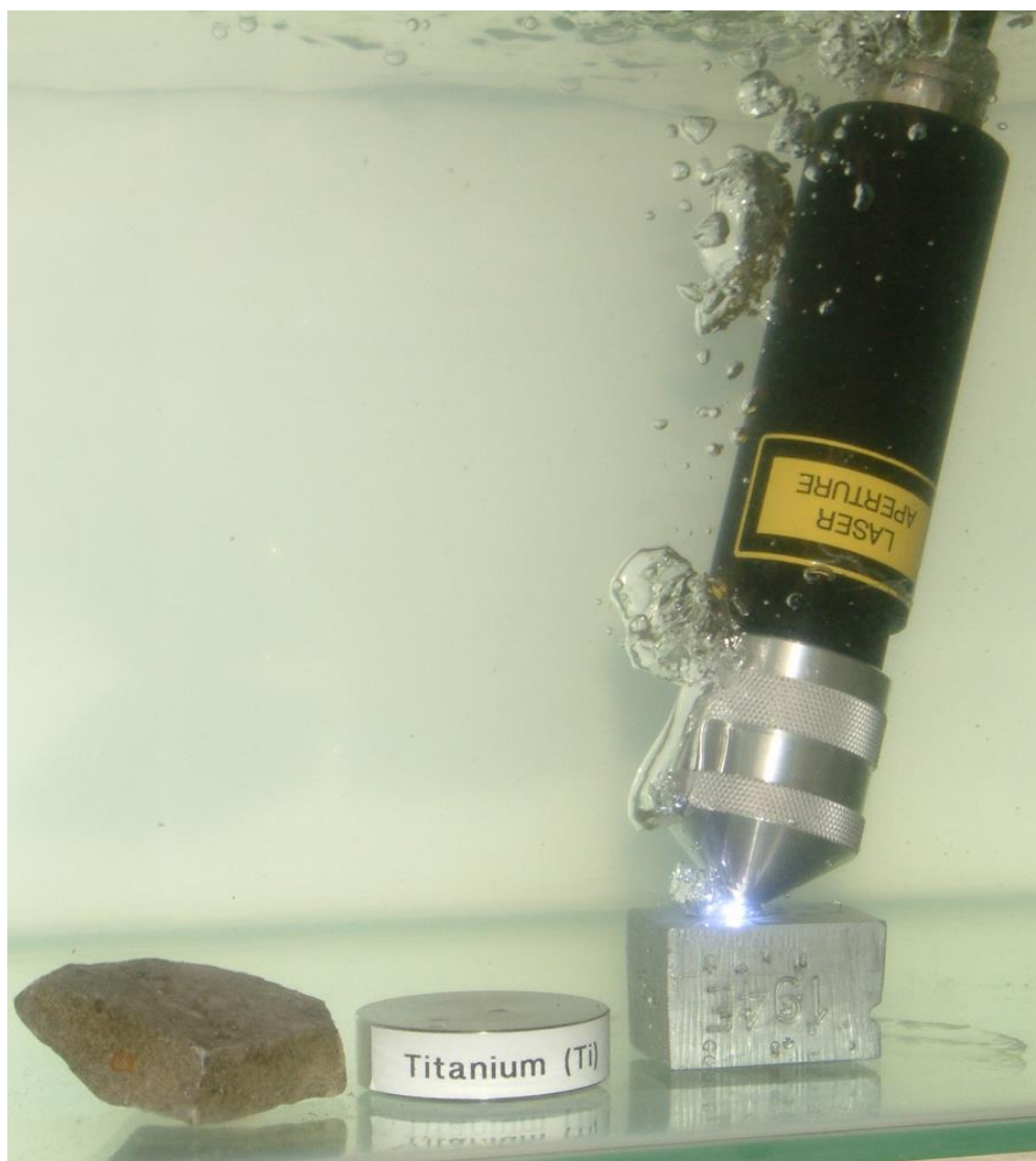
APL's submersible FO-LIBS probe being used to analyse objects submerged in water
