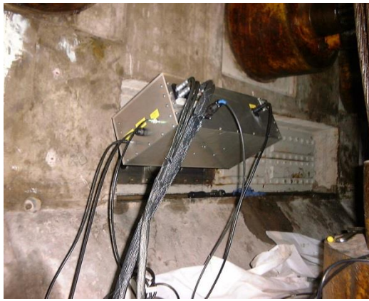
ST-LIBS module attached to pressure vessel wall using mechanical attachment to bolt anchor points
