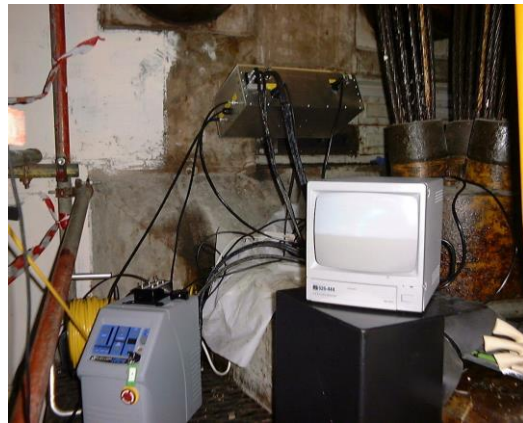
ST-LIBS module attached to pressure vessel wall using mechanical attachment to bolt anchor points
